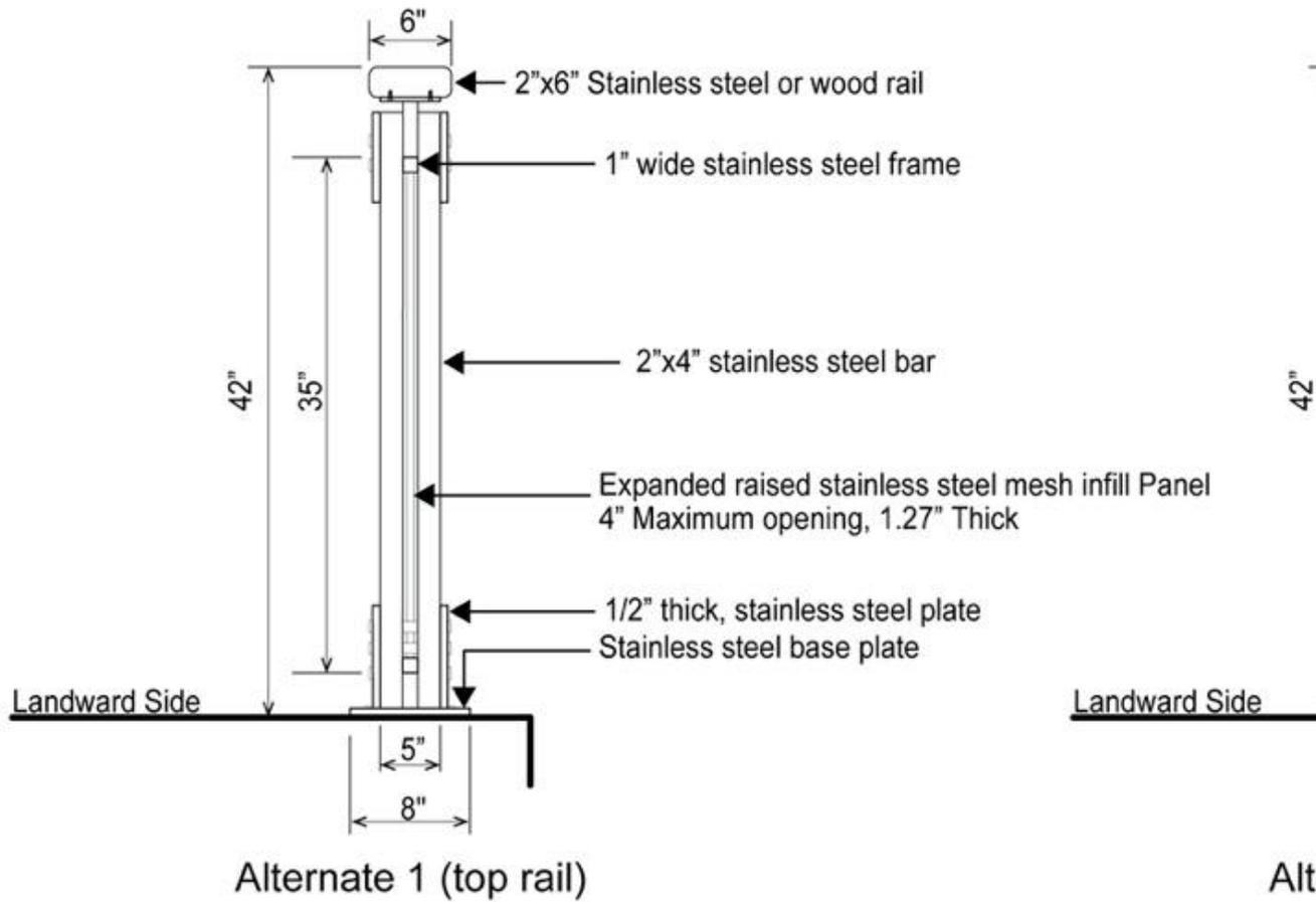
All guardrail components and hardware shall be in unpainted stainless steel and shall conform to any additional standards set forth by DPR.
