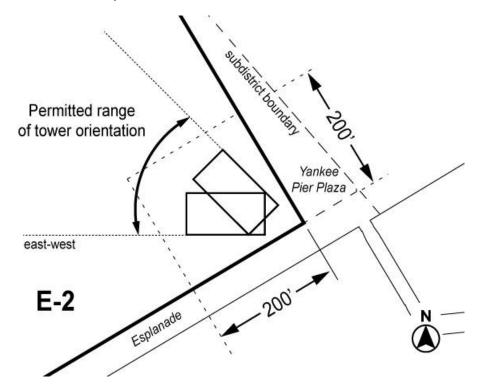
On the portion of #building parcel# E-2 that is beyond 200 feet of #Yankee Pier Plaza#, and on #building parcels# E-3 and E-4, for portions of #buildings# above a height of 125 feet, the provisions of paragraph (a) of this Section shall apply where no #story# within such portion has a gross area greater than or equal to 20,000 square feet, and the provisions of paragraph (b) shall apply where any #story# within such portion has a gross area greater than 20,000 square feet.
