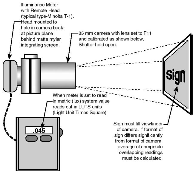
The LUTS meter must be calibrated prior to use. Although the lens is nominally set to F11, the actual light transmission value may differ especially with long focal length zoom lenses
