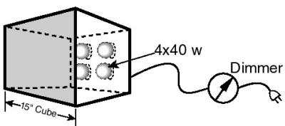
To calibrate, build a lightbox as shown above. The front of the box shall be 1/4" #2447 opal plexiglass; the other five interior sides shall be painted matte white.
