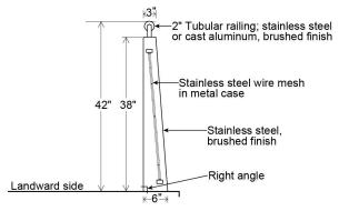
GUARDRAIL WITH METAL TOP Side Elevation
