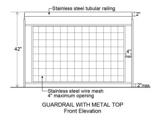
All guardrail components and hardware shall be in No. 316 Stainless Steel, passivated and bead blasted.
